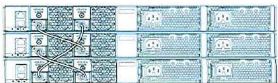
Figure 11: Example of a Data Stack with Full Bandwidth Connections
